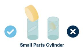
Place the toy or any removable component of a toy intended for children under 3 years of age, without compressing it and in any orientation into the small parts cylinder. If the toy or removable component fits entirely within the cylinder, it fails to comply with standards for children under 3 years of age.
