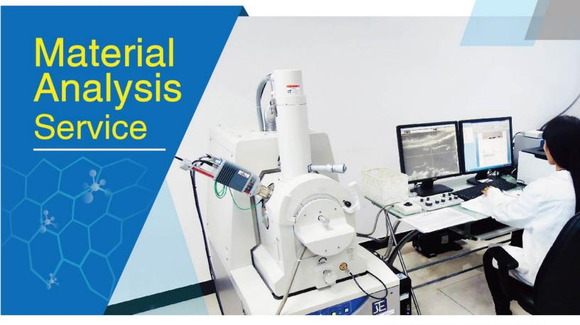
Scanning Electron Microscope (SEM) is a type of electron microscope that produces images of a sample by scanning the surface with a focused beam of electrons. The electrons interact with atoms in the sample, producing various signals that contain information about the sample's surface topography, construction and composition.
